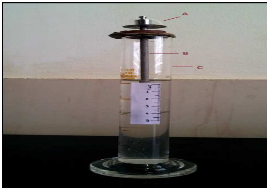
Figure No.1: Gel Strength measuring device (A) Weights (B) Device (C) Graduated cylinder (D) gel
